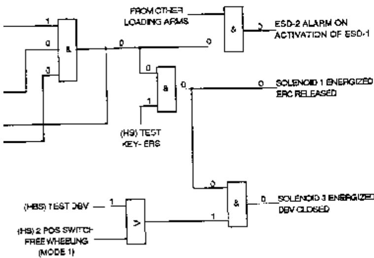
b) AUTOMATIC ACTIVATION OF ERS BY OVEREXTENSION OF SLEWING AND/OR APEX ANGLE STILL POSSIBLE
